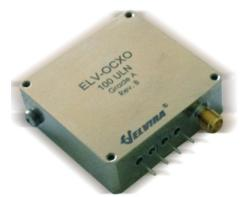
The ELV-OCXO 100 ULN is a high performance oven controlled crystal oscillator which features excellent frequency stability and ultra low single sideband phase noise. The oscillator provides more than +18 dBm of output power and draws 250 mA in the steady state from a +15V power supply. It comes in a compact aluminum milled form factor and operates over the frequency range of  $0...+50^{\circ}C$
